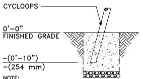
CONCRETE FOOTING AND NO. 4 REBAR (BY OTHERS) PER LOCAL SOIL CONDITIONS. CONSULT PROJECT ENGINEER FOR EXACT REQUIREMENTS.
